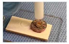
• The back plate is gently pushed down with a finger onto the stem.
